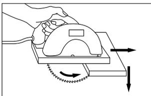
For best results when using an electric circular or jig saw, cut the Tandem surfaces face down so that the saw teeth cut into the laminate surface starting from the profiled front edge.
