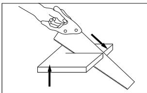
If using a hand saw, (10 to 12 teeth per 25mm) cut the Tandem surfaces face up. Always start from the profiled front edge and keep the saw at a low angle.
